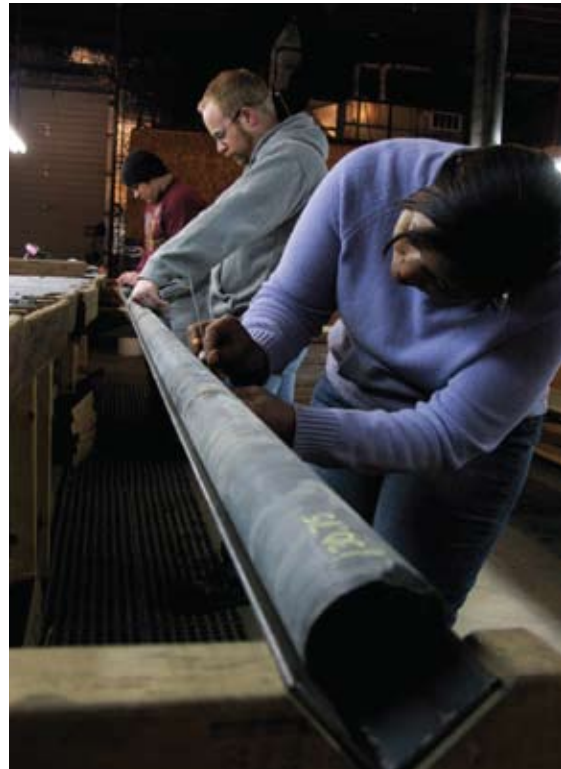
Field geologists (Cody Suits, Jason Evans, Joanne Scott) examine core samples in order to determine mineral content at the Kennecott Eagle Minerals Company in Marquette.
