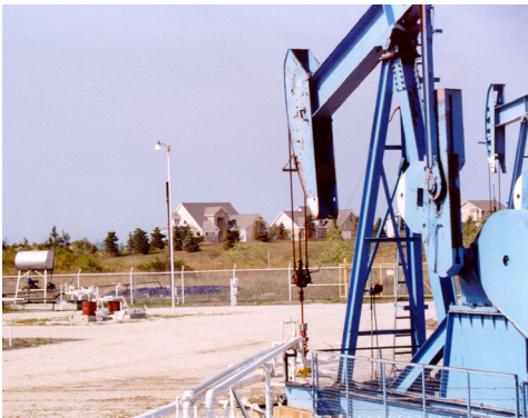
Prior to the ban, this derrick, which operated near the shore of Lake Michigan in Muskegon, safely extracted oil from beneath the lake through a directional pipeline running under a multi-million dollar residential development.
