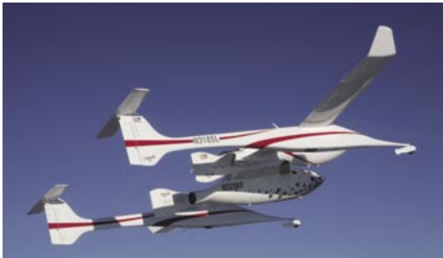
The privately funded SpaceShipOne is shown here underneath White Knight, the plane that launches the ship into space. Photo courtesy of Scaled Composites
